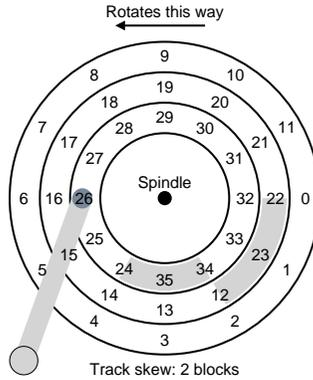
Figure 37.4: **Three Tracks: Track Skew Of 2**
