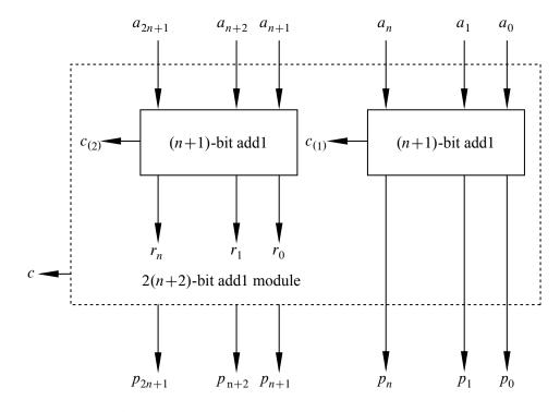
Figure 3.1 Structure of a Double-size *add1* Module.
