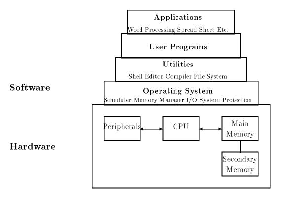
Figure 1.1: Computer System Block Diagram
